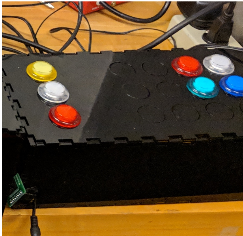
Figure 38: Shielded control box with arcade style buttons.
