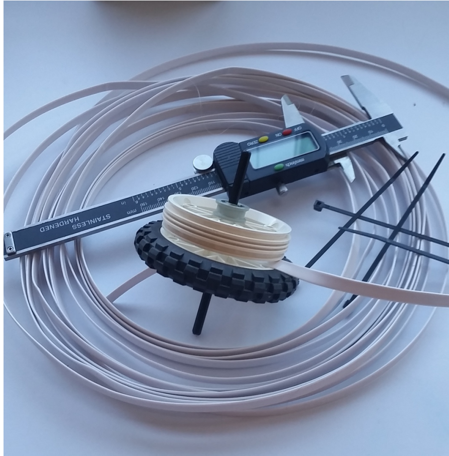
Figure 33: LEGO Mindstorms-based coil-winding jig.
