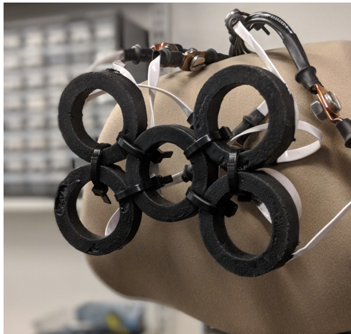
Figure 35: H bridge array in vehicle headrest orientation.
