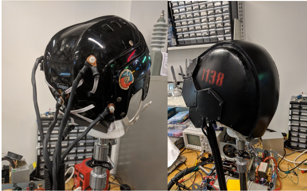
Figure 36: Wearable array with isolation hood for dark adaptation.
