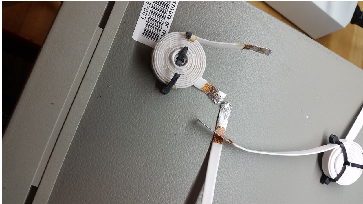
Figure 25: Initial 30mm Litz wire test coils.
