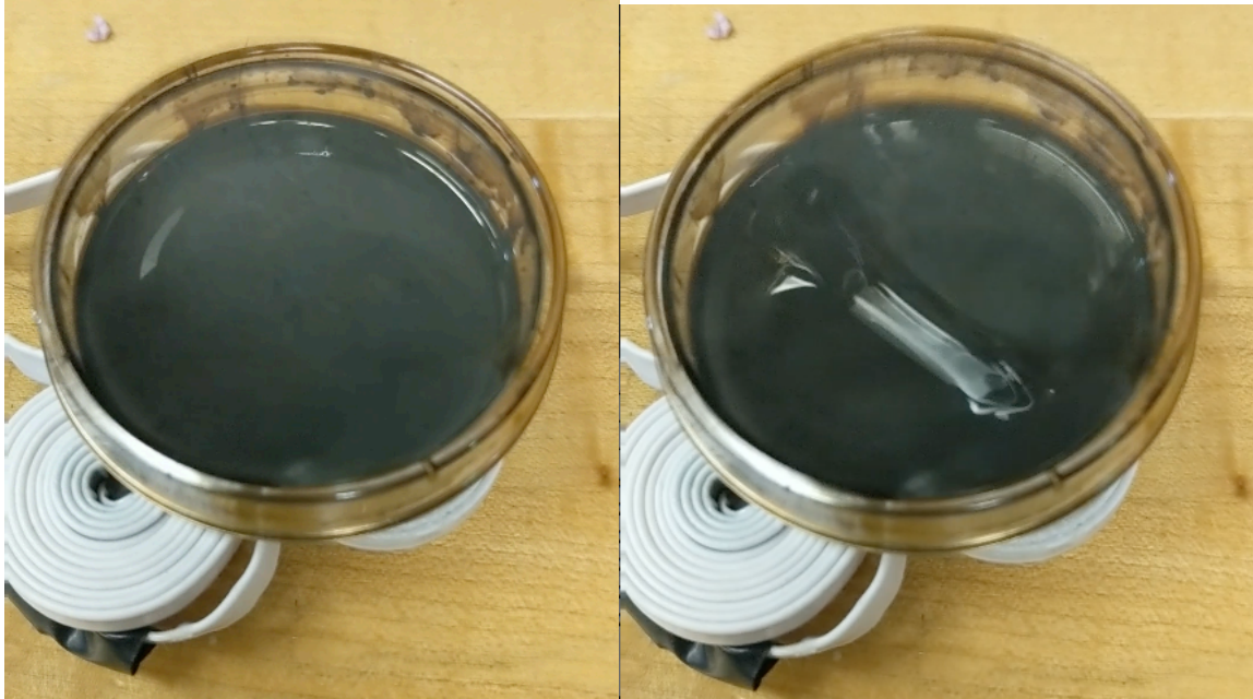
Figure 27: Ferrofluid visualization of butterfly focality filmed at 120fps (8.33ms).
