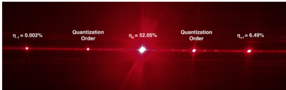
Figure 4. Bragg grating characterization with laser beam incident at Bragg angle and resulting asymmetric diffraction profile, depicting very strong energy transfer into the +1st diffracted order at the expense of energy transferred into other orders.
